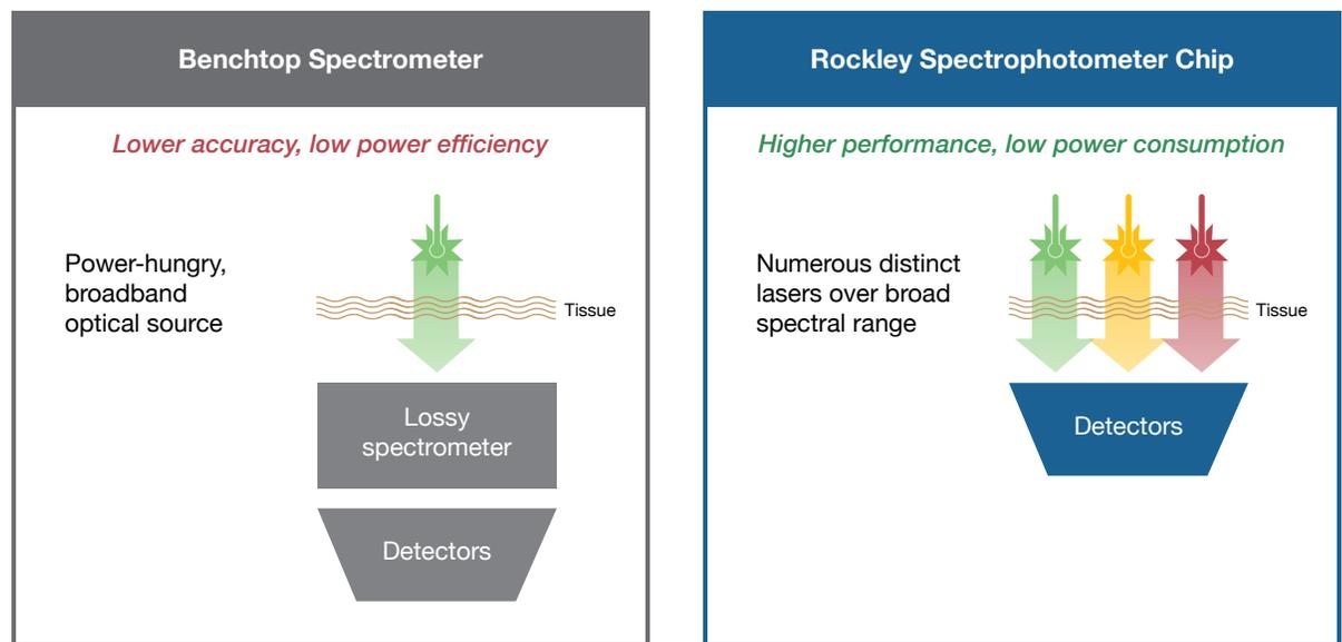
Figure 4: Comparison of benchtop spectrometer to Rockley’s spectrophotometer chip
