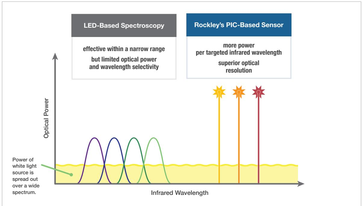
Figure 5: Rockley spectrophotometer chip solution, as compared to conventional LED- and spectrometer-based solutions
