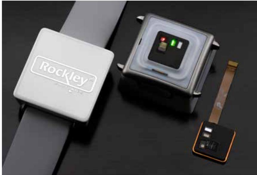
*Figure 3: Rockley wristband with standalone sensor module containing photonic ICs and application firmware*
