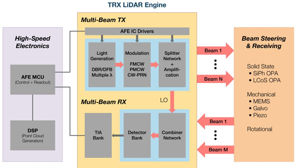
Figure 3: Block diagram of components needed, both optical and IC, to build a LiDAR engine.
