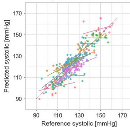
Figure 5. Basic linear model systolic predictions on 20 hold-out subjects with individual subject colors and best-fit lines. Only the Rockley laser signal information and a single calibration measurement was utilized. No heart rate or demographic information is utilized.
