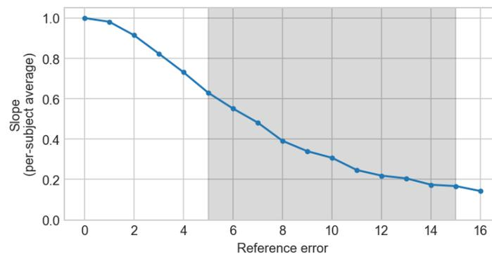
Figure 8. Simulated per-subject average slope as a function of increasing reference error. The simulation is based on 100 subjects, each with 15 blood pressure reference readings. The shaded area indicates the expected reference error from cuff-based measurements as compared to arterial in-line pressure sensors.
