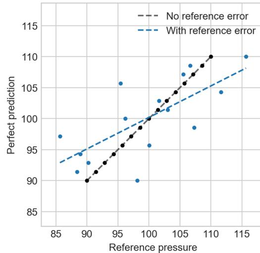
Figure 7. Scatter plot illustrating regression dilution. A perfect prediction with no error is plotted versus reference readings with no error (black dots, black dashed regression line) and with 5 mmHg random error (blue dots, blue dashed regression line). When error is introduced to the reference readings, the slope of the regression line is reduced.
